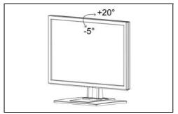
Grasp the monitor with both hands on the right and left edge of the casing and adjust it to the desired rake.
